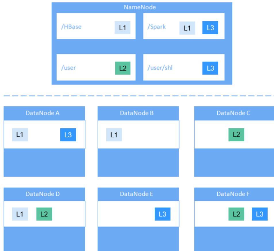
Figure 1-53 Example of label-based block placement policy
